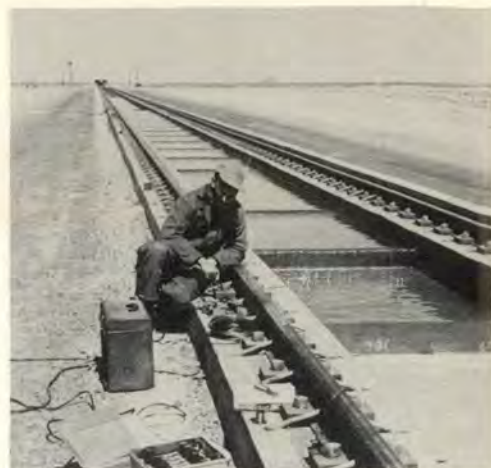
Small plastic dams hold the desired water level for braking action of high speed sled.
