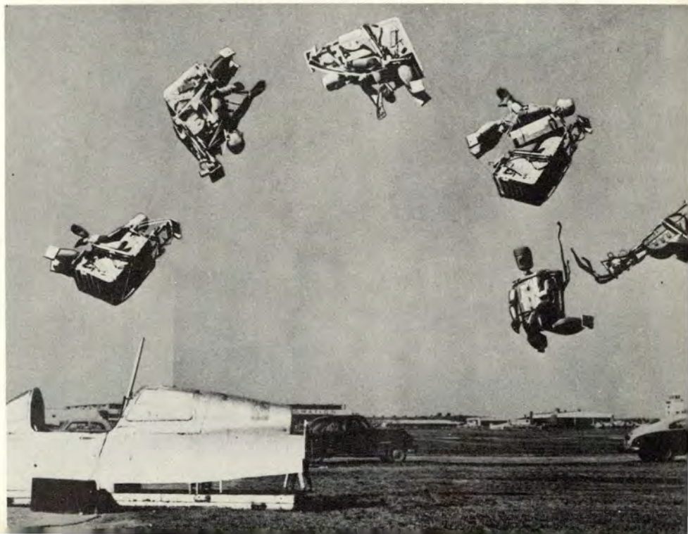
A new pilot-ejection seat developed by Republic is tested in composite picture below. The seat has a device which automatically disconnects the safety belt at the peak of the arc after ejection.
