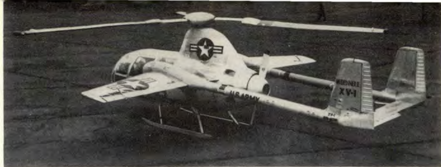
The Convertiplane embodies a new concept of flight, the unloaded rotor. This revolutionary aircraft is equipped with a rotor for vertical flight, and wings and a prop for horizontal flight.
